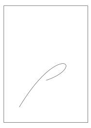
The operation <code>-bez23</code> is a shorthand used when the first control point is equal to the current point. The operation <code>-bez13</code> is a shorthand used when the second control point is equal to the final point.
