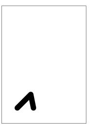
The miter limit (see PDF reference for details) may be set with -miter.
